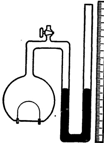
FIG. 99.—Air-thermometer ammeter
