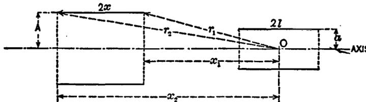
FIG. 203.—Coaxial solenoids not concentric
