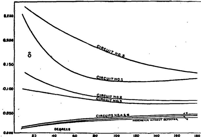
FIG. 74.—Increase in decrement of the wave-meter circuit due to the detector circuit
