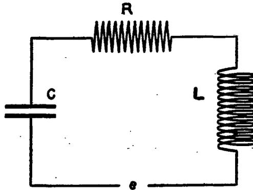
FIG. 10.—Circuit with resistance, inductance, and capacity in series; a typical radio circuit
