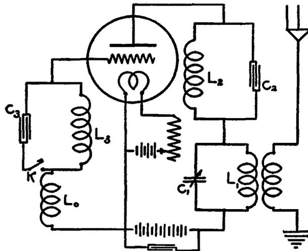
FIG. 157.—Method of coupling tone-circuit generator to an antenna
