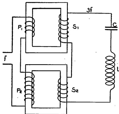
FIG. 165.—Use of two transformers for producing frequency transformations
