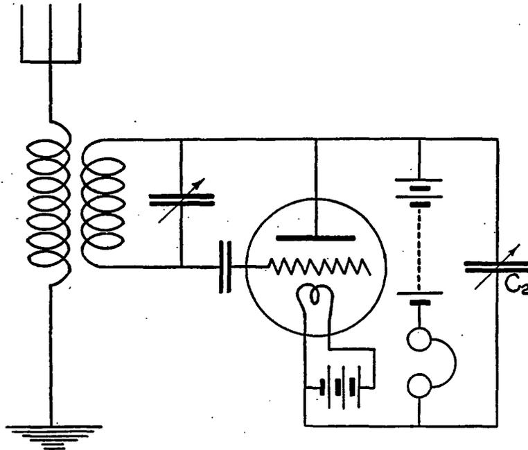
FIG. 152.—“Ultraudion” circuit for receiving undamped oscillations
