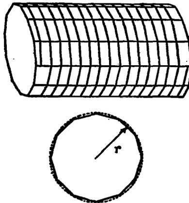
FIG. 182.—Polygonal coil
