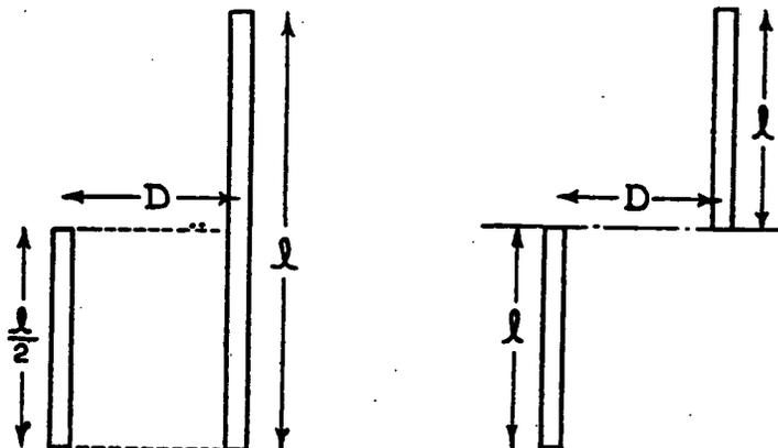
FIG. 195.—Two wires with axes in parallel. FIG. 196.—Two wires with axes in parallel lines, lines; another particular case of Fig. 193 with one end of each on the same perpendicular
