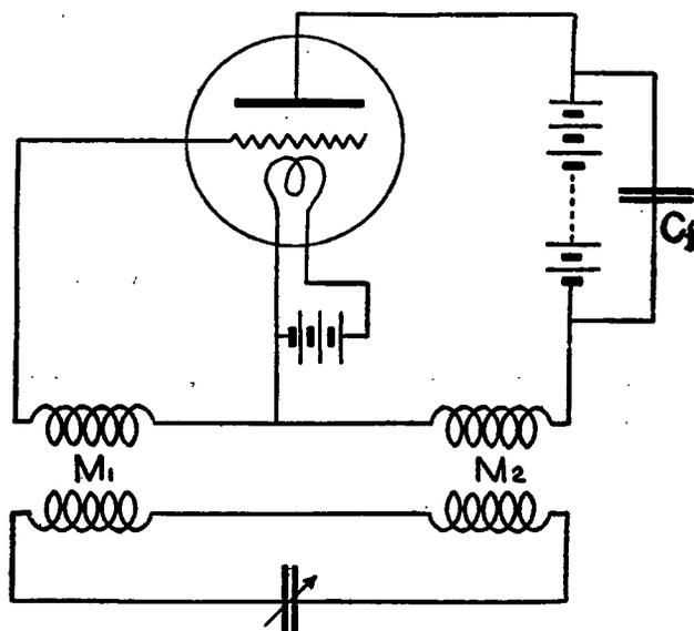
FIG. 147.—Generating circuits in which the oscillatory circuit is inductively coupled to both the grid and plate circuits
