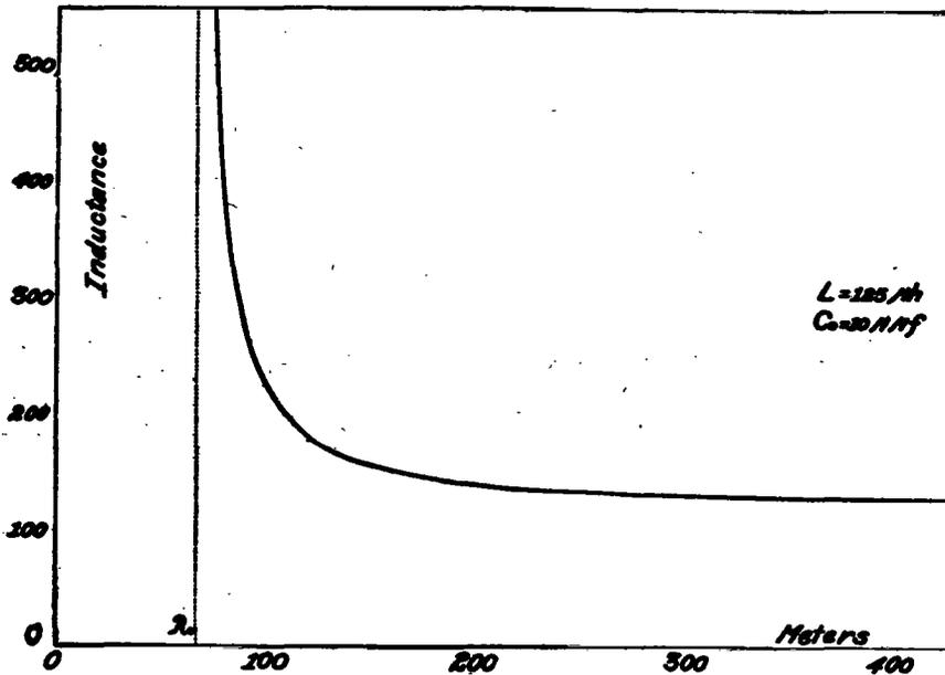
FIG. 48.—Variation of apparent inductance of a coil with wave length
