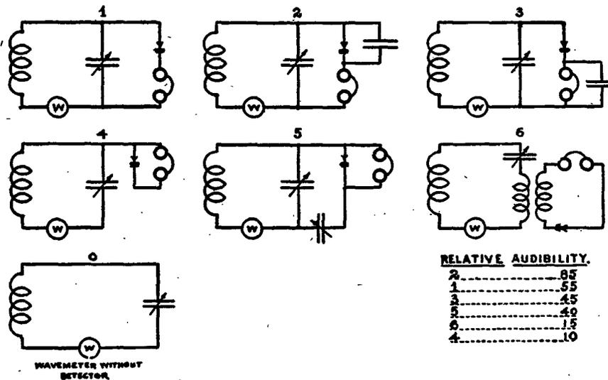
FIG. 72.—Various wave-meter circuits, using detector and phones
