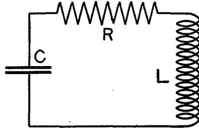
FIG. 66.—Oscillatory circuit having resistance, inductance, and capacity in series
