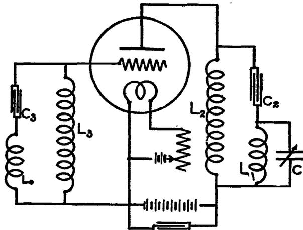
FIG. 156.—Arrangement for producing modulated radio-frequency current by use of a single tube
