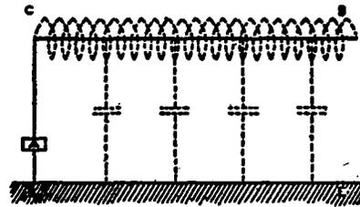
FIG. 59.—Antenna with uniformly distributed capacity and inductance
