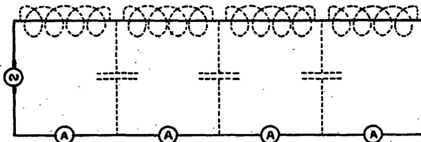
FIG. 54.—Circuit representing distributed capacity and inductance
