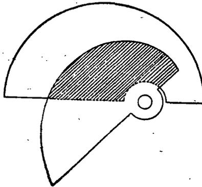
FIG. 82.—Form of rotary condenser plates in which the per cent change of capacity is the same throughout the entire range of the condenser
