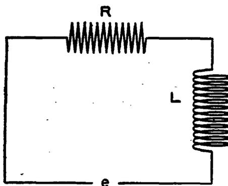
FIG. 9.—Circuit with resistance and inductance in series
