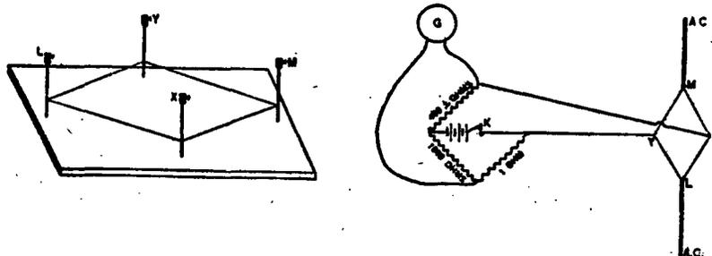
FIG. 124.—Standard ammeter using the bolometer principle
