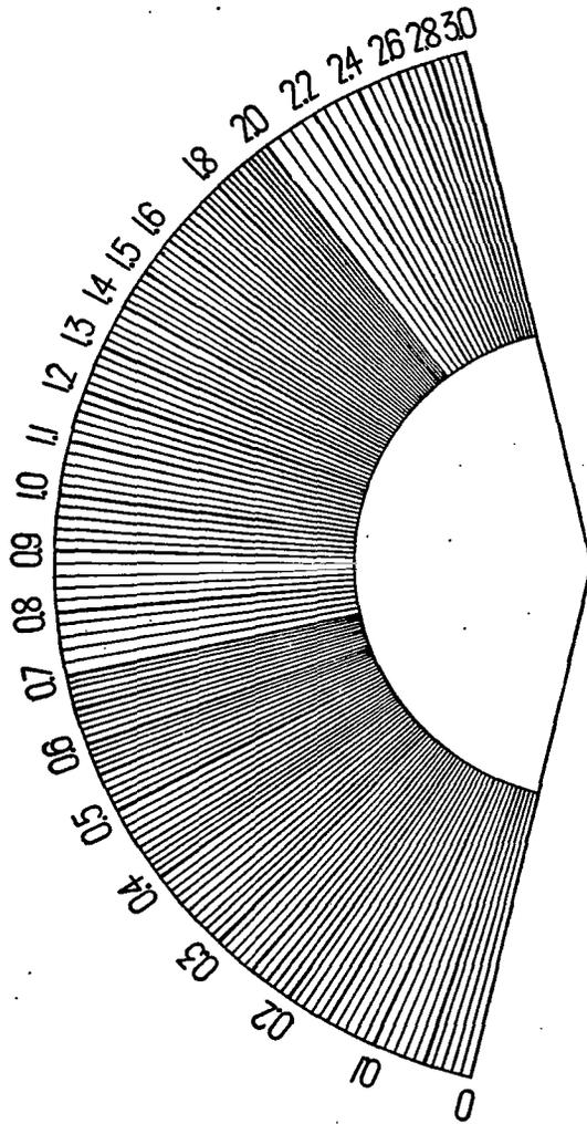
FIG. 135.—*Direct-reading decrement scale for any semicircular-plate condenser*
