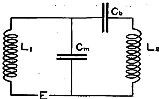
FIG. 34.—Special case of capacitive coupling
