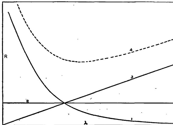
FIG. 64.—Variation of antenna resistance with wave length
