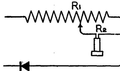
FIG. 119.—Circuit for measuring audibility ratios
