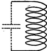
FIG. 45.—Circuit which is equivalent to a coil having distributed capacity
