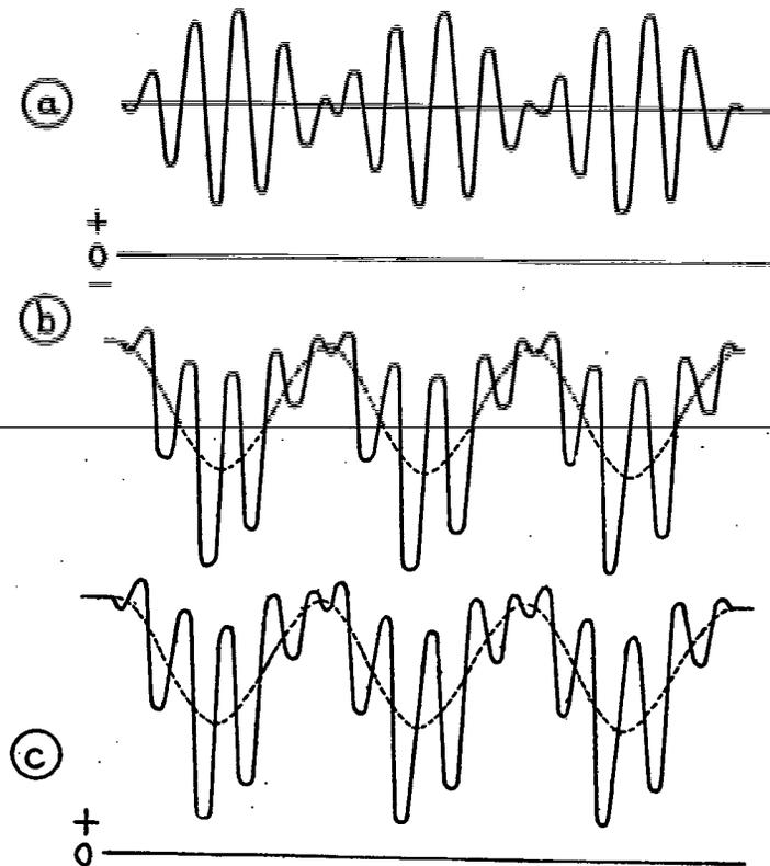
FIG. 151.—Variations of mean grid voltage and mean plate current as beat oscillations are being produced
