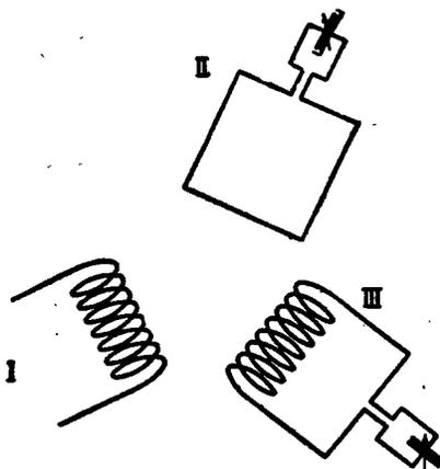
FIG. 71.—Circuits involved in the comparison of inductance standards
