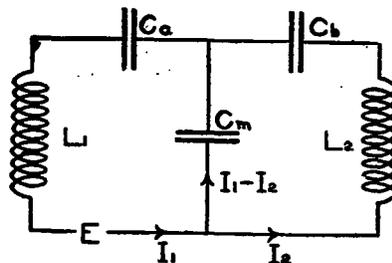
FIG. 41.—Circuits involving capacitive coupling
