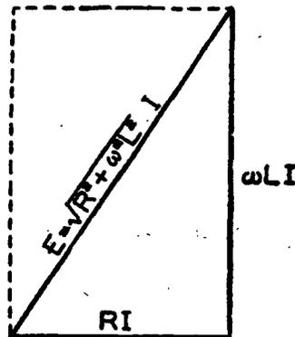
FIG. 12.—Vector combination of electromotive forces
