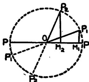
FIG. 7.—Successive positions of revolving conductor; the emf generated is proportional to the sine of the angle formed by the revolving conductor and POP
