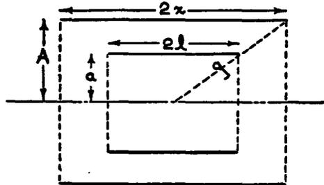
FIG. 205.—Coaxial concentric solenoids, outer coil being longer
