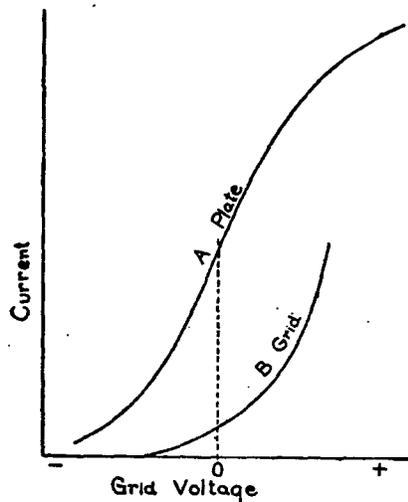
FIG. 136.—Variation of plate current (usually in milliamperes) and grid current (usually in microamperes) with grid voltage
