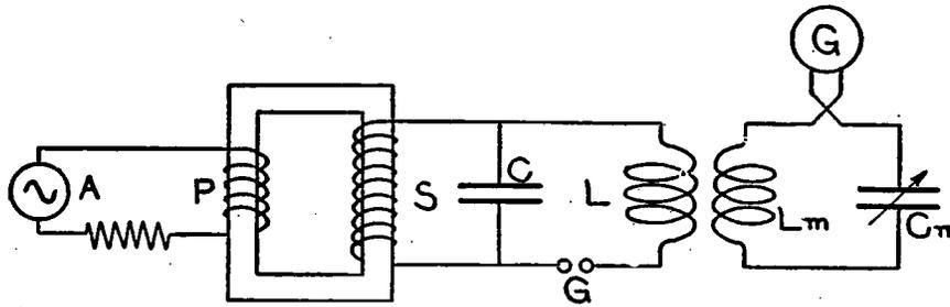
FIG. 168.—Typical spark circuit for producing high-frequency oscillations
