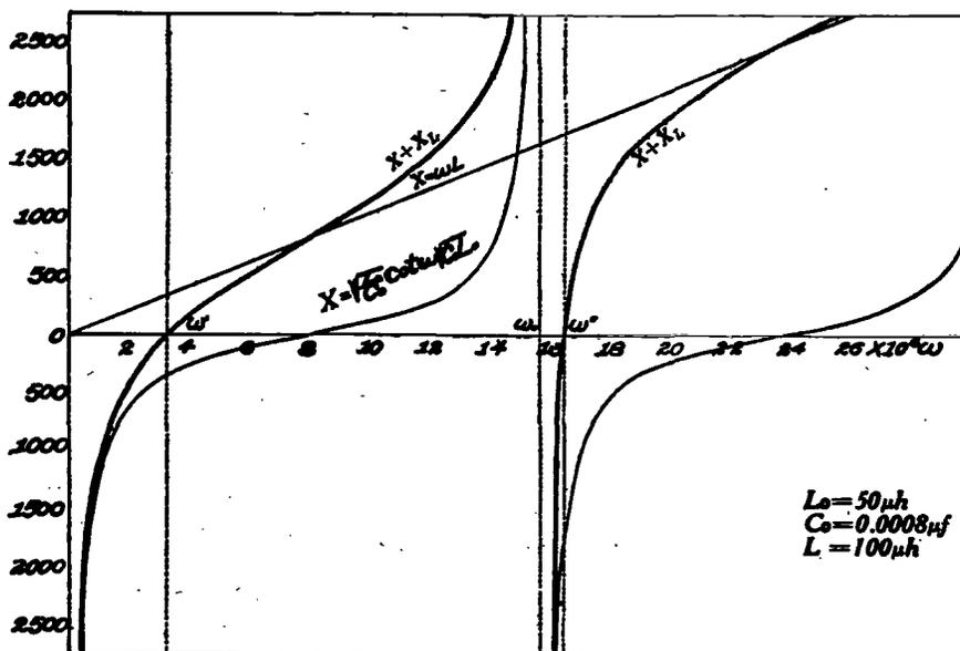
FIG. 62.—Reactance curve for antenna with series inductance
