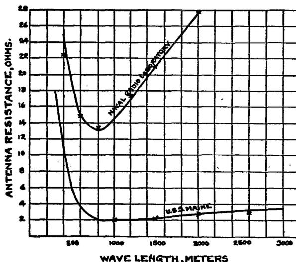
FIG. 91.—Variation of antenna resistance with wave length
