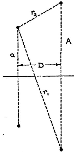
FIG. 199.—Cross sections of two parallel coaxial circles
