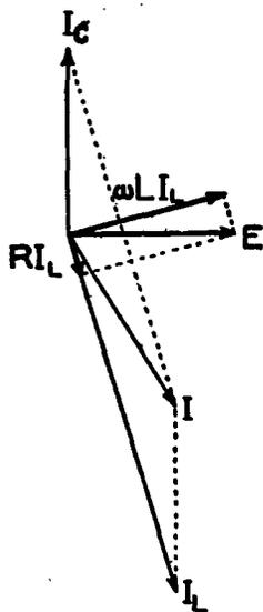
FIG. 22.—Vector diagram for parallel circuit
