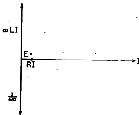
FIG. 18.—*Vector diagram of series circuit in resonance*
