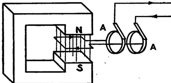
The simplest type of dynamo generates an alternating current
