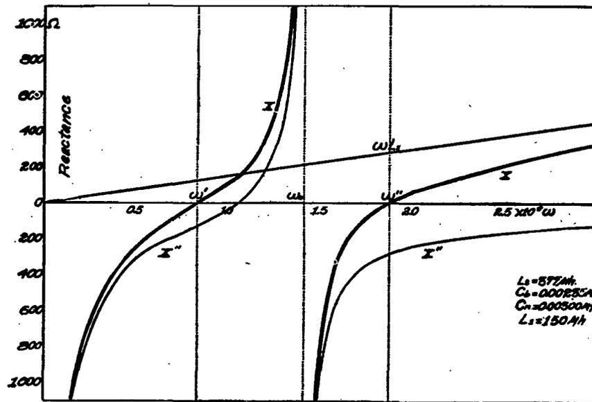
FIG. 35.—Reactance diagram for case of capacitive coupling shown in Fig. 34
