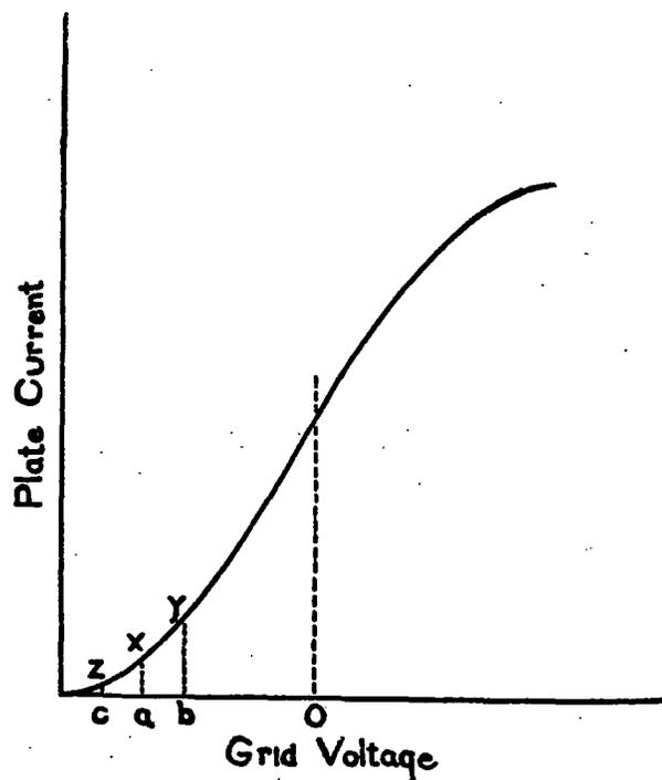
FIG. 139.—Plate characteristic, showing region of curve where rectifying action is large
