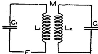
FIG. 38.—Circuits involving inductive coupling
