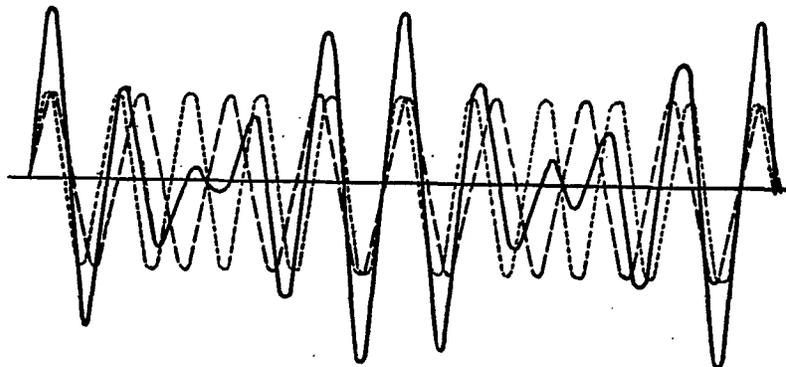
FIG. 150.—Mode of adding component oscillations
