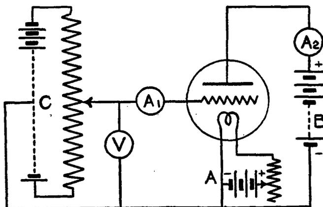
FIG. 137.—Scheme of connections for determining characteristic curves
