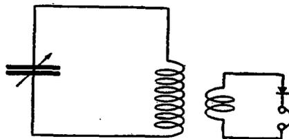
FIG. 76.—Arrangement of circuits for determining resonance by coupling to an aperiodic detector circuit
