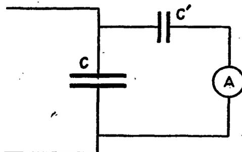
FIG. 105.—Capacity shunted ammeter
