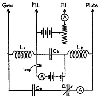
FIG. 160.—Scheme of connections for pliotron generator
