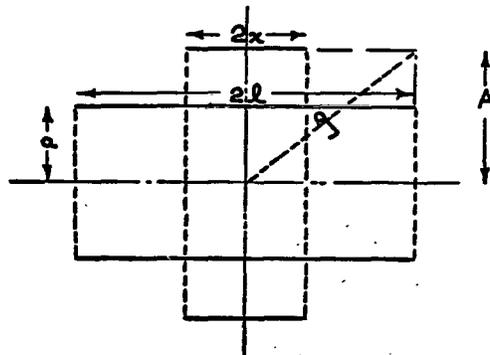
FIG. 206.—Coaxial concentric solenoids, outer coil being shorter
