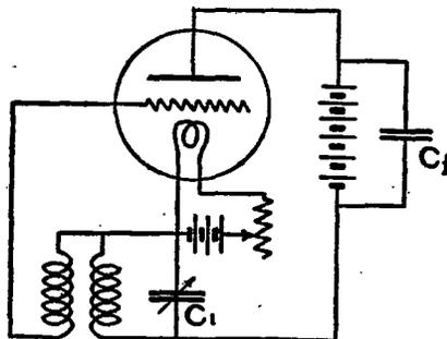
FIG. 146.—Use of electron tube as a generator
