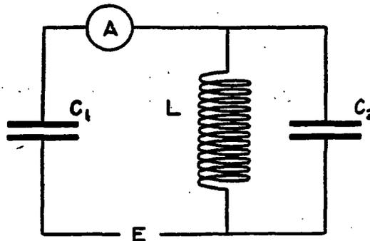
FIG. 29.—Simple case of coupled circuits in which a parallel circuit is combined with a series circuit
