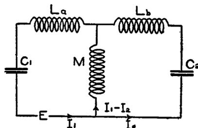
FIG. 36.—Circuits involving direct coupling
