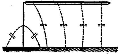
FIG. 58.—Form of antenna of large capacity
