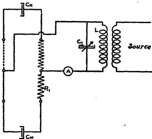
FIG. 132.—Circuit for precision measurement of condenser resistance with switching device and small tuning condenser
