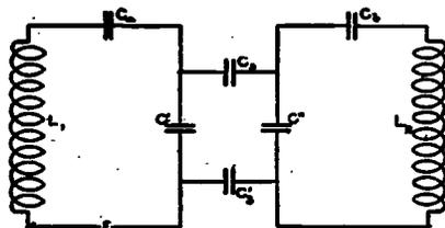
FIG. 43.—Generalized case of capacitive coupling
