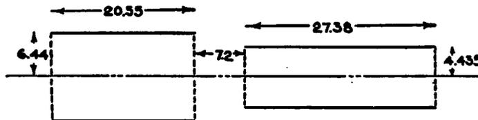
FIG. 204.—Example of coaxial solenoids not concentric
