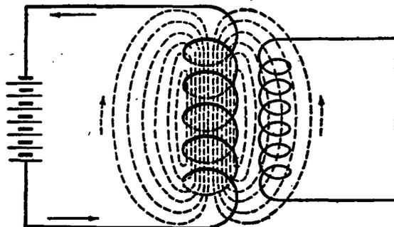
FIG. 5.—Linking of magnetic flux of one circuit with another; the basis of the conception of mutual inductance
