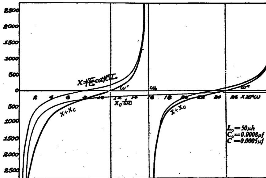
FIG. 63.—Reactance curve for antenna with series condenser
