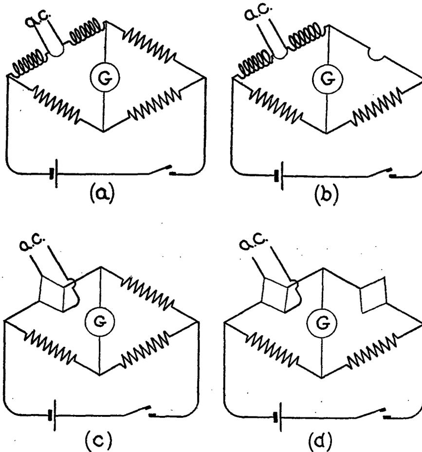
FIG. 114.—Various methods of using the bolometer for measuring small radio currents
