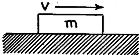
FIG. 4.—A body having a mass ( $m$ ) and a velocity ( $v$ ) opposes any change in its momentum ( $mv$ )
