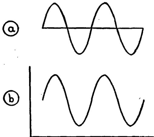
FIG. 144.—Variations of plate current with grid voltage
