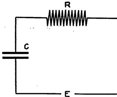
FIG. 11.—Circuit with resistance and capacity in series
