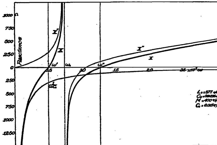
FIG. 33.—Reactance diagram for the simple coupled circuits of Fig. 31; the curve  $X$  of resultant reactance is zero for two values of frequency
