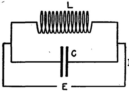
FIG. 27.—Simple parallel circuit
