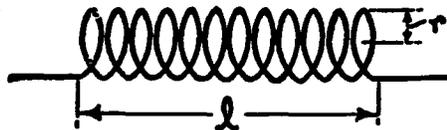
FIG. 2.—Simple solenoid
