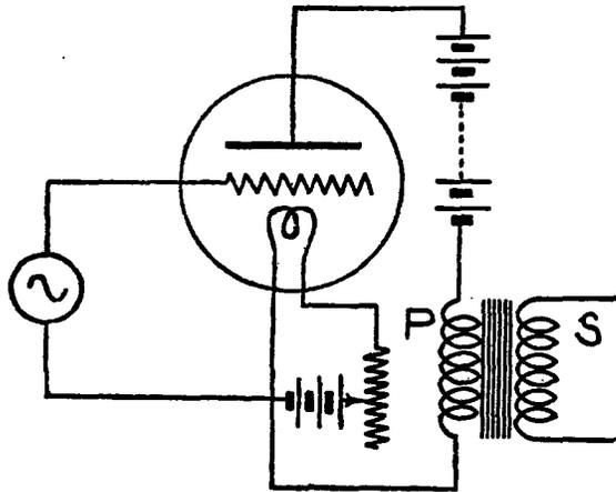
FIG. 143.—Use of electron tube as an amplifier
