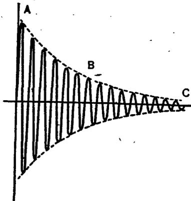
FIG. 67.—Wave train with a logarithmic decrement of 0.2
