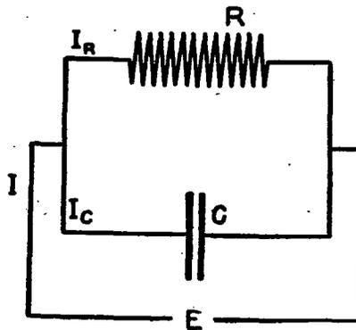
FIG. 15.—Circuit with resistance and capacity in parallel
