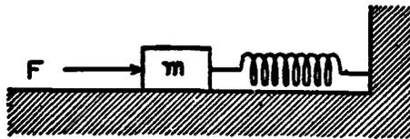
FIG. 17.—Simple mechanical system which can exhibit the phenomenon of resonance
