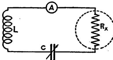
FIG. 126.—Method of measuring resistance by calorimeter method
