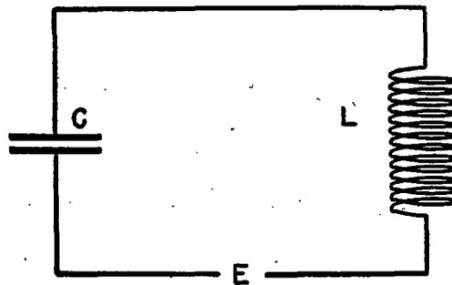
FIG. 25.—Simple series circuit
