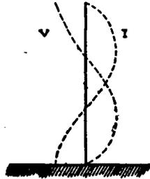
FIG. 57.—The distribution of current and voltage in the simple antenna when oscillating in the first harmonic
