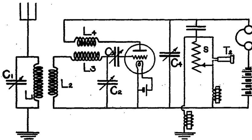
FIG. 122.—Oscillating audion circuits for quantitative measurements on undamped waves from distant radio stations
