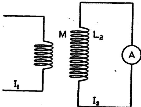
FIG. 106.—Inductance shunted ammeter inductively coupled. Principle of the current transformer
