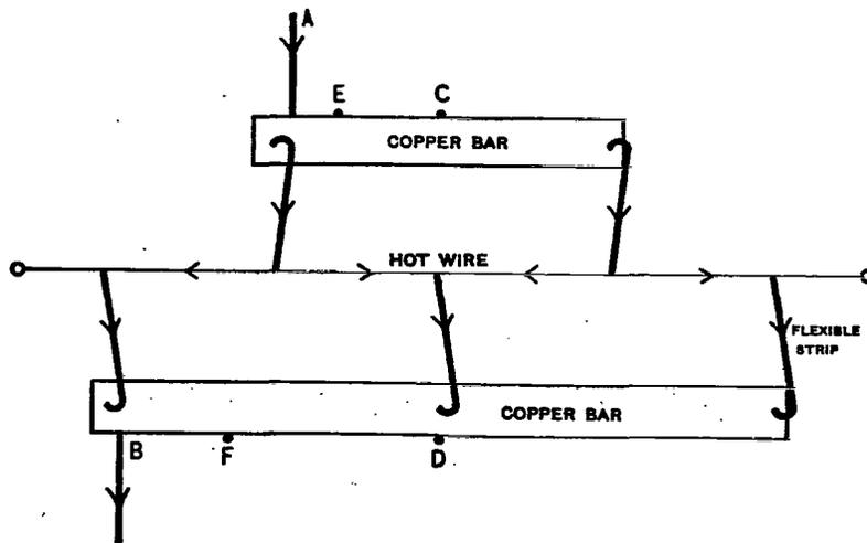
FIG. 103.—*So-called unshunted ammeter of four sections*
